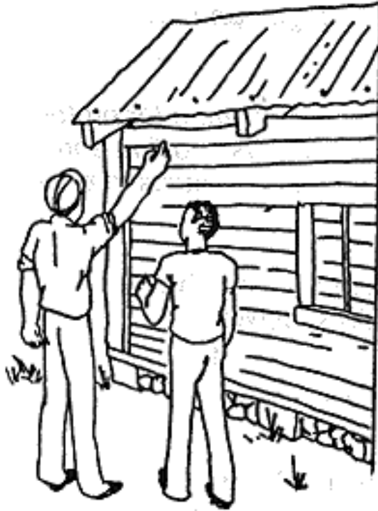
Do not leave too much space between the roof and the walls!
